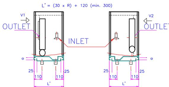
Standard-evaporating coil type DX with driptray
